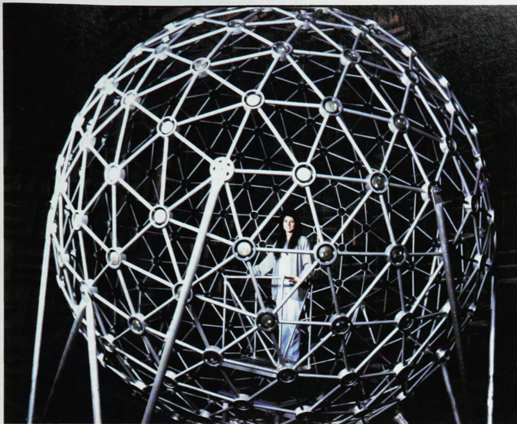
FIGURE 1. THE SOUND LOCALIZATION FACILITY at Wright Patterson Air Force Base in Dayton, Ohio, is a geodesic sphere, nearly 5 m in diameter, housing an array of 277 loudspeakers. Each speaker has a dedicated power amplifier, and the switching logic allows the simultaneous use of as many as 15 sources. The array is enclosed in a 6 m cubical anechoic room: Foam wedges 1.2 m long on the walls of the room make the room strongly absorbing for wavelengths longer than 5 m, or frequencies above 70 Hz. Listeners in localization experiments indicate perceived source directions by placing an electromagnetic stylus on a small globe. (Courtesy of Mark Ericson and Richard McKinley.)
